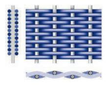
HOLLANDER (DUTCH) WEAVE is made with relatively thin weft wires packed closely together, and thicker more widely spaced warp wires. It resembles a 'basket' weave and does not have square apertures. Dimensionally very stable and having high bursting strength, it is suitable for pressure filtration where a large open area is not required.
