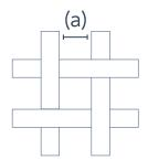
APERTURE SIZES Our standard filter cloths range from 2,000 micron to 3 micron aperture, the measurement being made across the square between the insides of adjacent threads, as shown.
