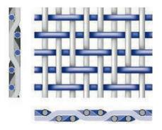
TWILL WEAVE is woven so that the individual wires in one direction pass over two and under the next two cross wires. It is less rigid than plain weave and is often used in very fine meshes.
