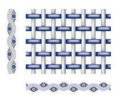
PLAIN WEAVE is woven from wires of the same diameter for both warp and weft, arranged in a symmetrical "over one and under one" pattern to provide square openings of precise dimensions. Plain mesh has great dimensional stability.
